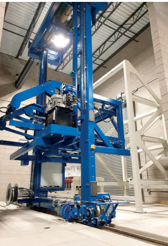
Automatic stacker crane that carries out the mold changes
