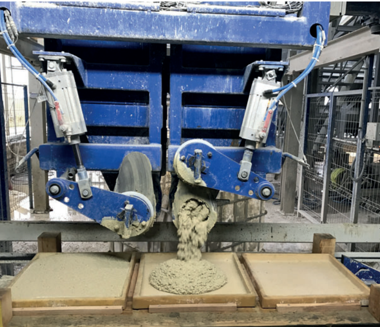
Fully automated dosing and filling system: quality, precision, cleanliness, versatility and flexibility
