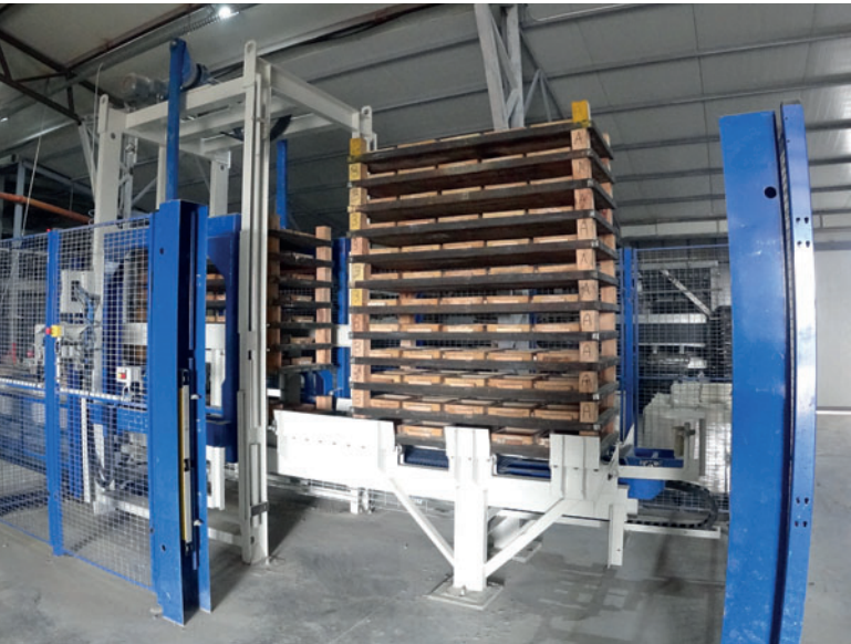
Elevator and lowerator: transfer and handling system provided by Quadra
