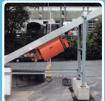
Rollover bucket in a 32° inclination = 60%
